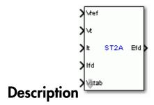
This block models a compound source rectifier excitation system. It utilizes both terminal voltage, Vt, and terminal current, It, to form a model of the exciter power source.
